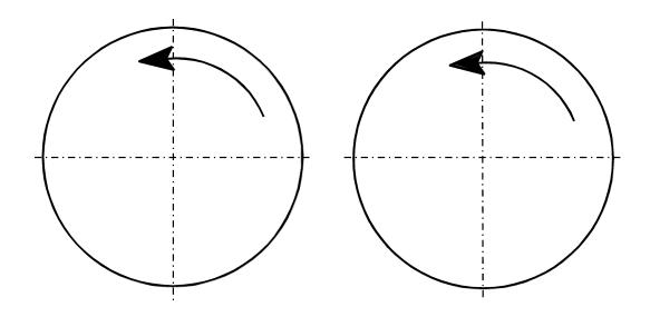
Figure 10 — Rollers with same direction of rotation
